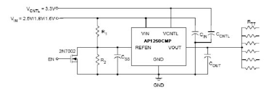
$R_1 = R_2 = 100 \text{K}\Omega$ ,  $R_{TT} = 50 \Omega/33 \Omega/25 \Omega$
